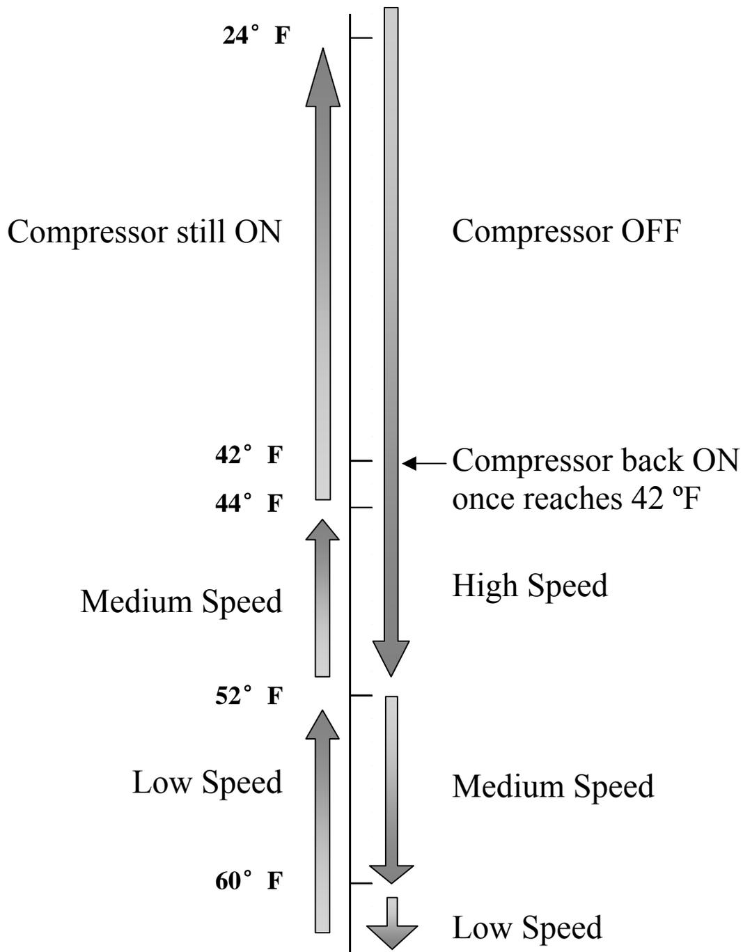
**Note: above diagram shows the compressor working schematic when 3 speed fan motor is used. For single speed fan motor only one speed is available.**
