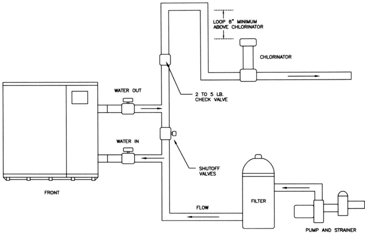
FIGURE 4 – PIPING CONNECTIONS
