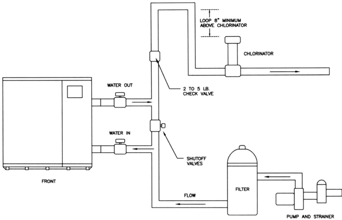
FIGURE 4 - PIPING CONNECTIONS
