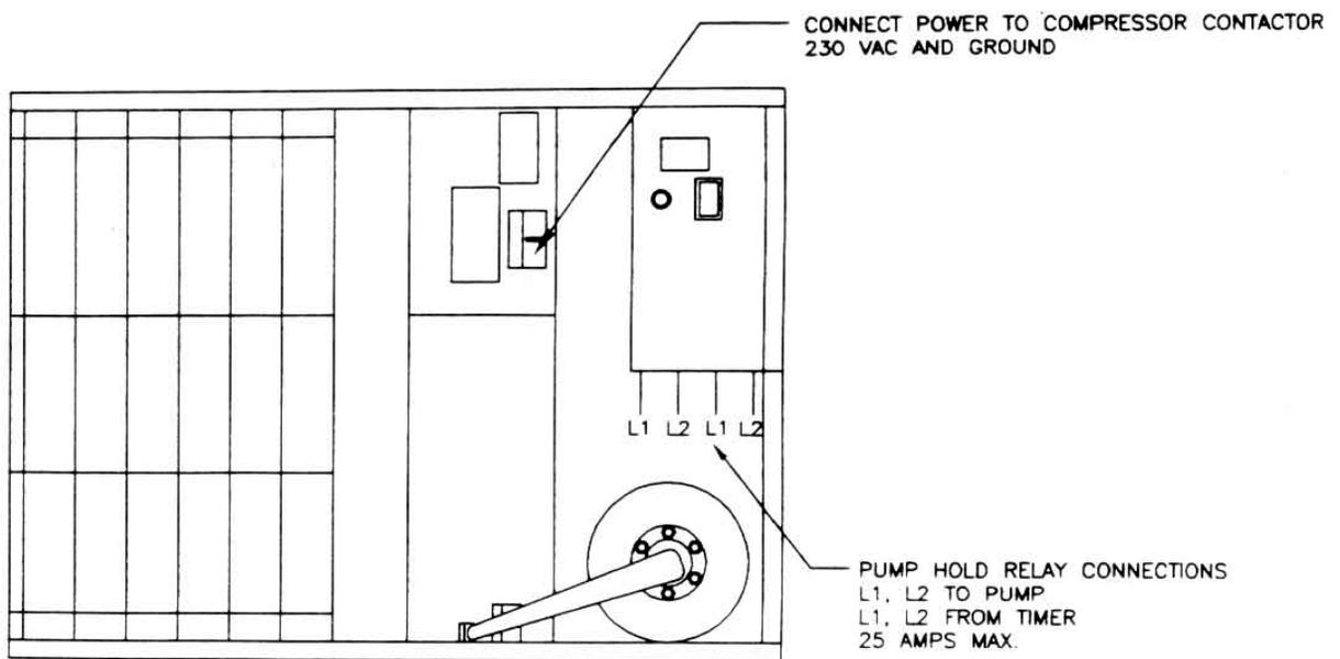
FIGURE 1 - ELECTRICAL CONNECTIONS
